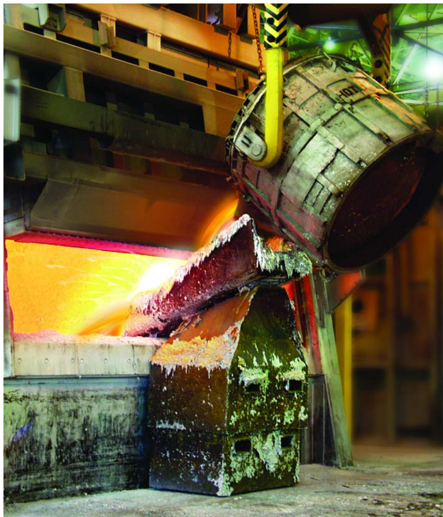
▲ Molten metal is poured from a crucible in the Ingot Department of the Alcoa plant.
